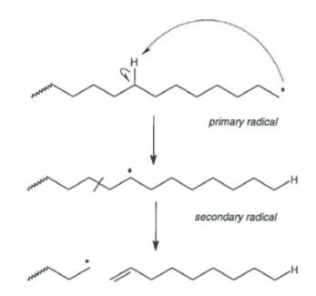
*Typical example of scission process in a polyolefine*
