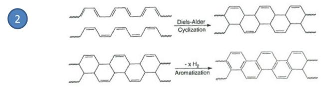
□ It means no fuel released in gas phase, except additives such plasticizers. At 2<sup>nd</sup> step, production of dihydrogene. After, oxidation of char due to oxygen diffusion, producing CO
