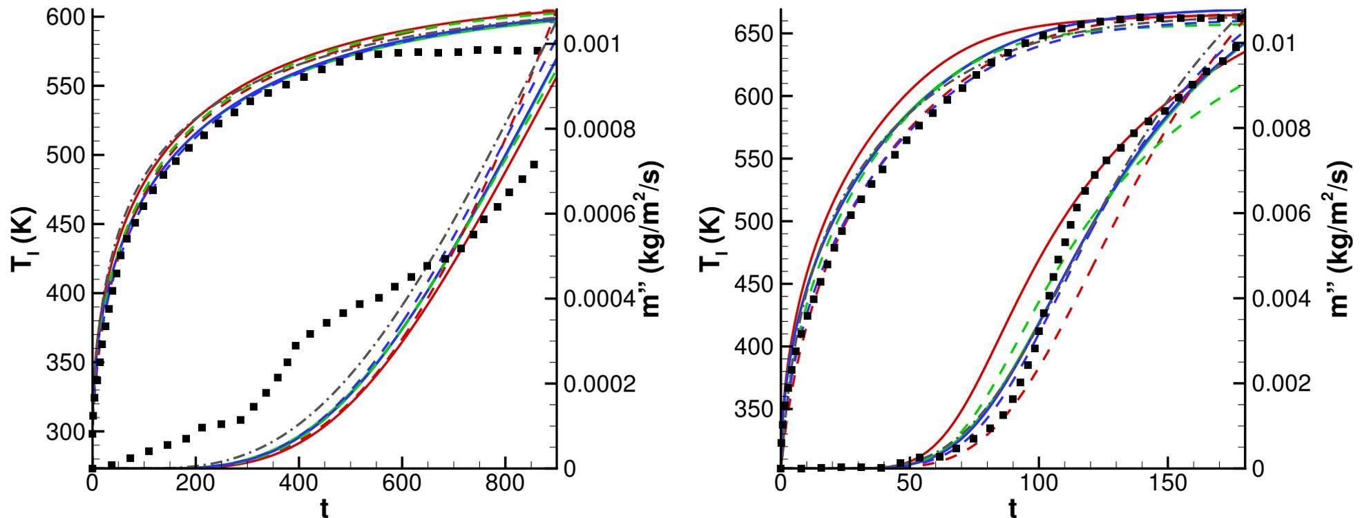
**Figure :** Comparison between the reference experimental results of Kashiwagi and Ohlemiller, 1982 (■) and the computed interface temperature ( $T_i$ ) and mass loss rate ( $\dot{m}''$ )
