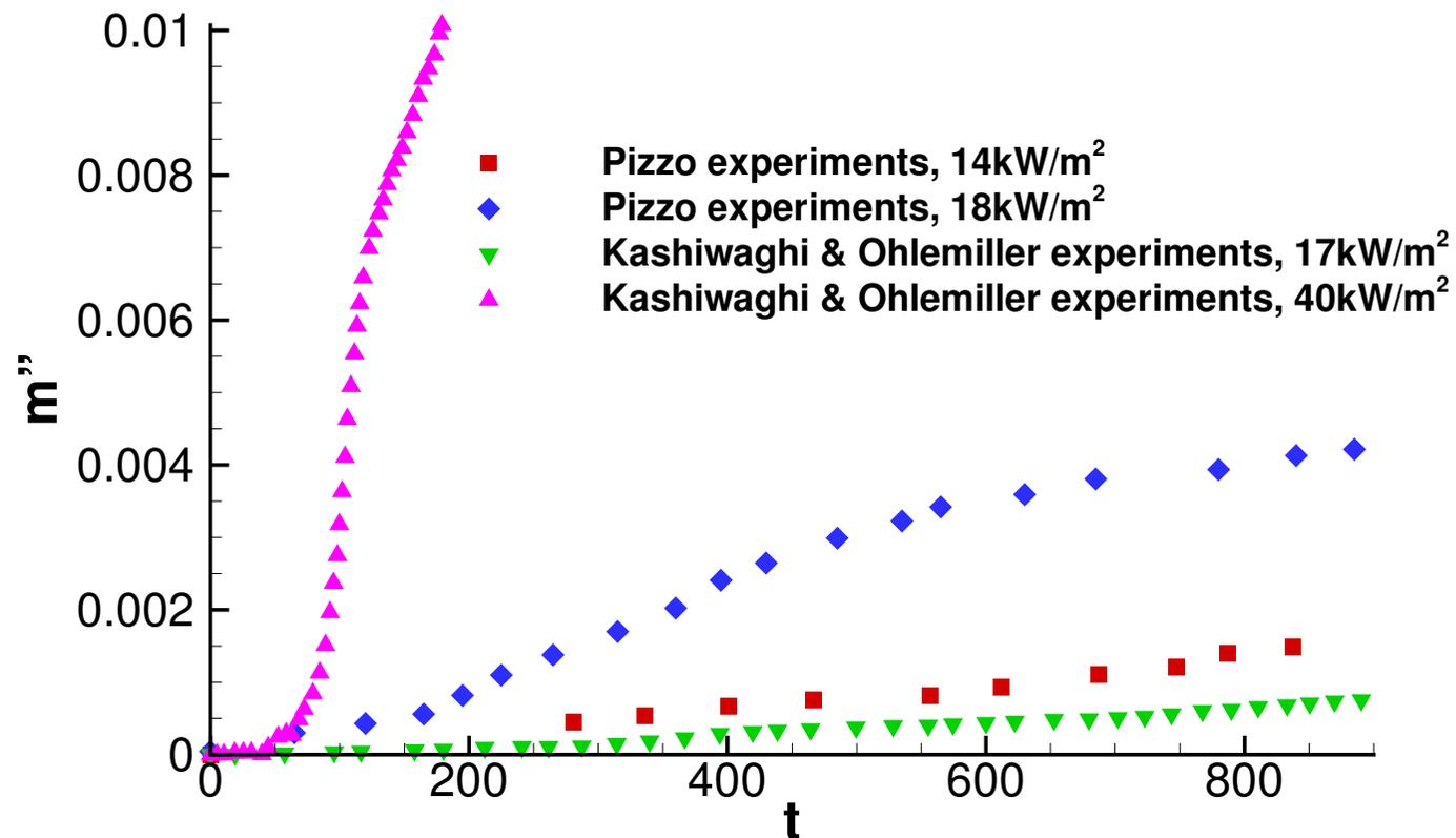
**Figure :** Mass loss rate evolution. Comparison between Kashiwagi & Ohlemiller and Pizzo Pizzo et al., 2015 experiments under 20% O<sub>2</sub>
