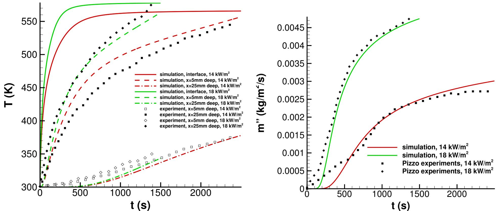
**Figure :** Comparison between the experimental results of Pizzo and the related simulations. Left: temperature; right: mass loss rate.
