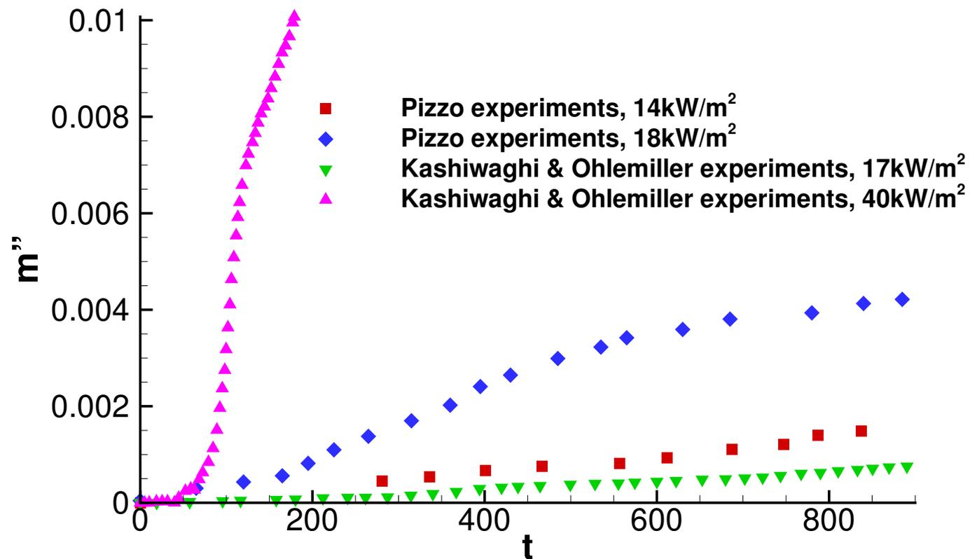
**Figure :** Mass loss rate evolution. Comparison between Kashiwaghi & Ohlemiller and Pizzo Pizzo et al., 2015 experiments under 20% O<sub>2</sub>
