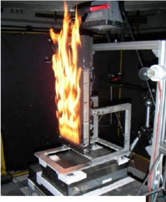
**Figure :** Flaming vertical PMMA flat plate
