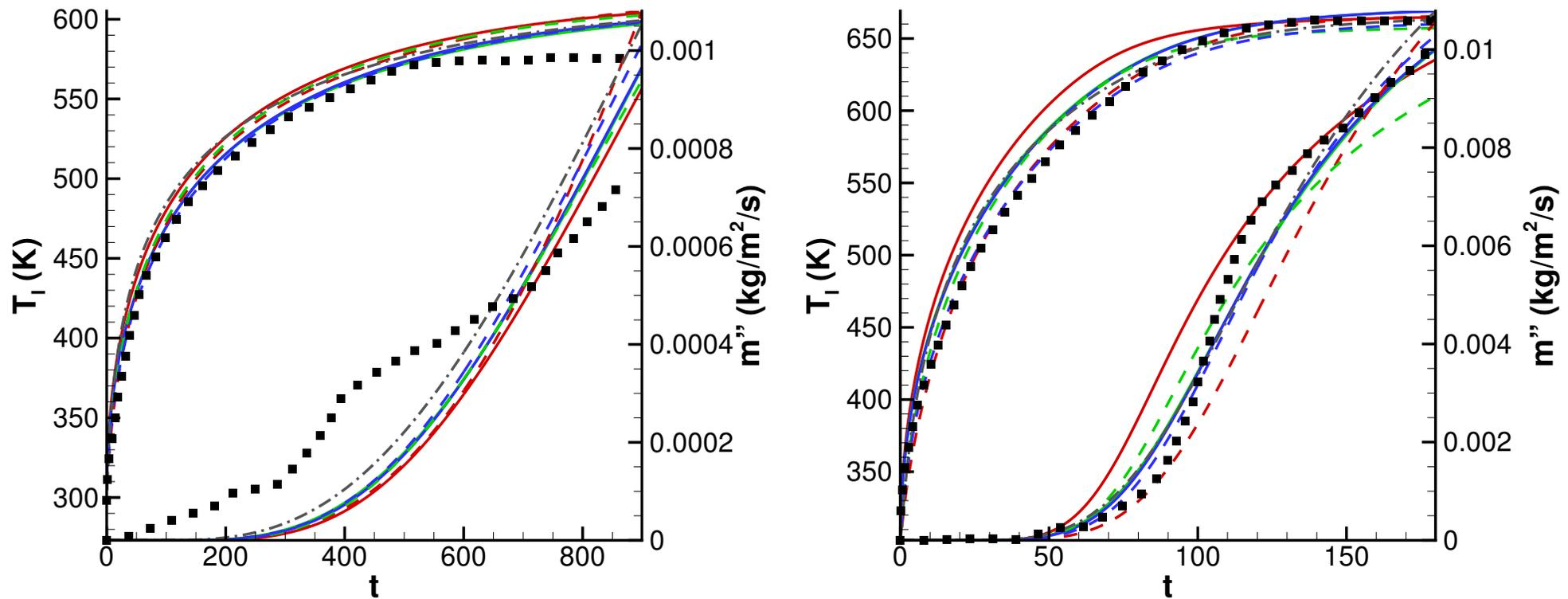
**Figure :** Comparison between the reference experimental results of Kashiwagi and Ohlemiller, 1982 (■) and the computed interface temperature ( $T$ ) and mass loss rate ( $\dot{m}''$ )
