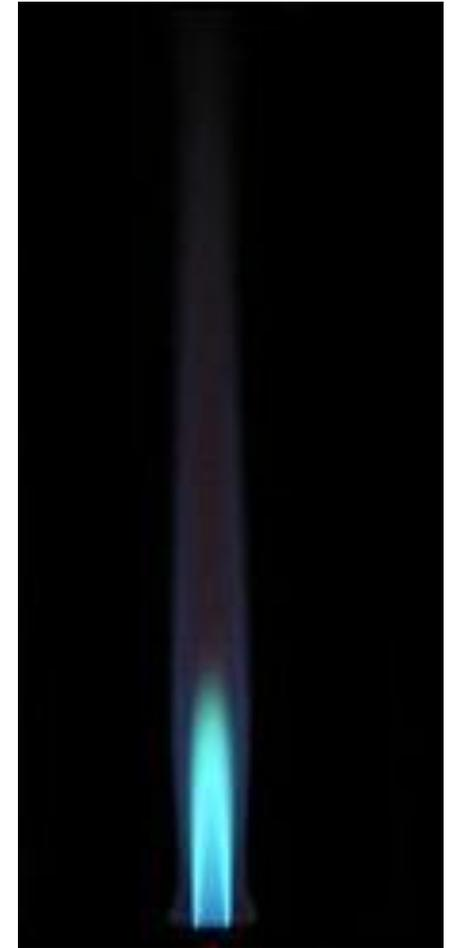
A premixed flame is a chemical reaction in which the fuel and the oxygen (oxidizer) are mixed before they burn.
