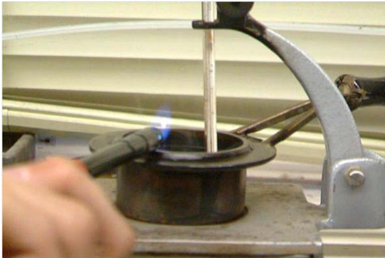
Cleveland Open Cup Tester (ASTM D92)
