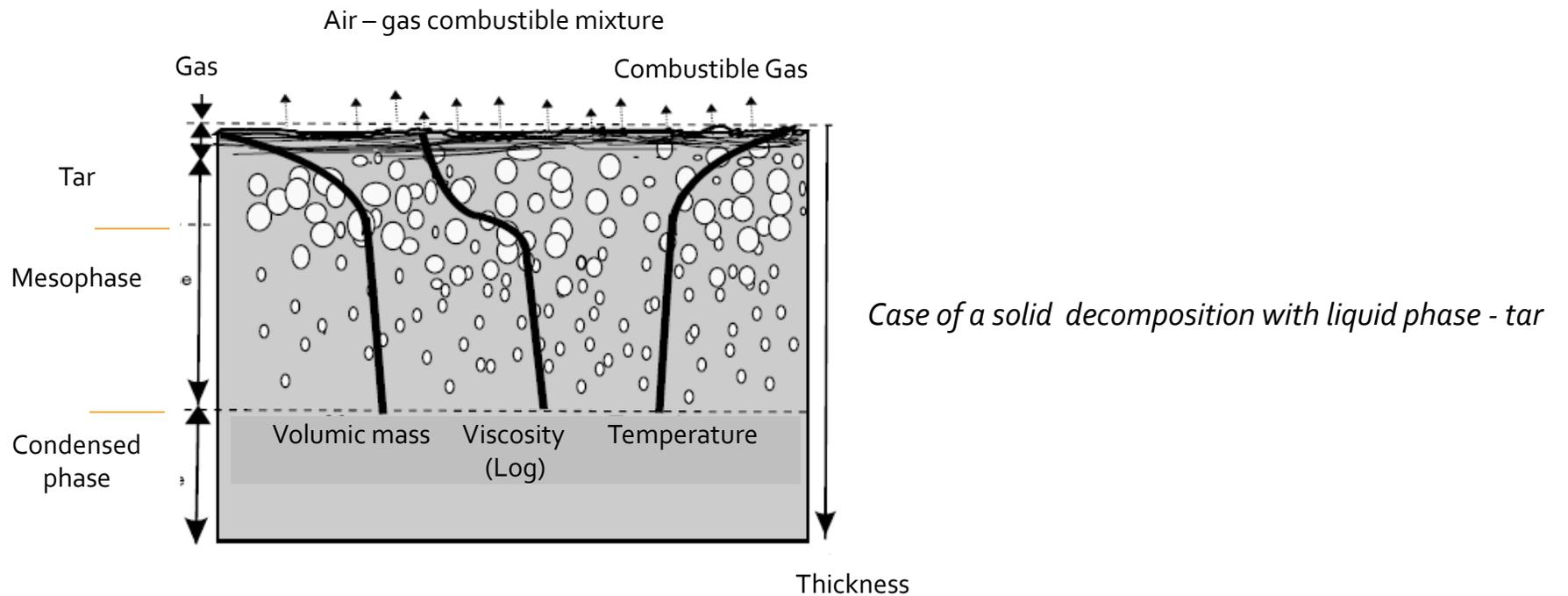
*Case of a solid decomposition with liquid phase - tar*
