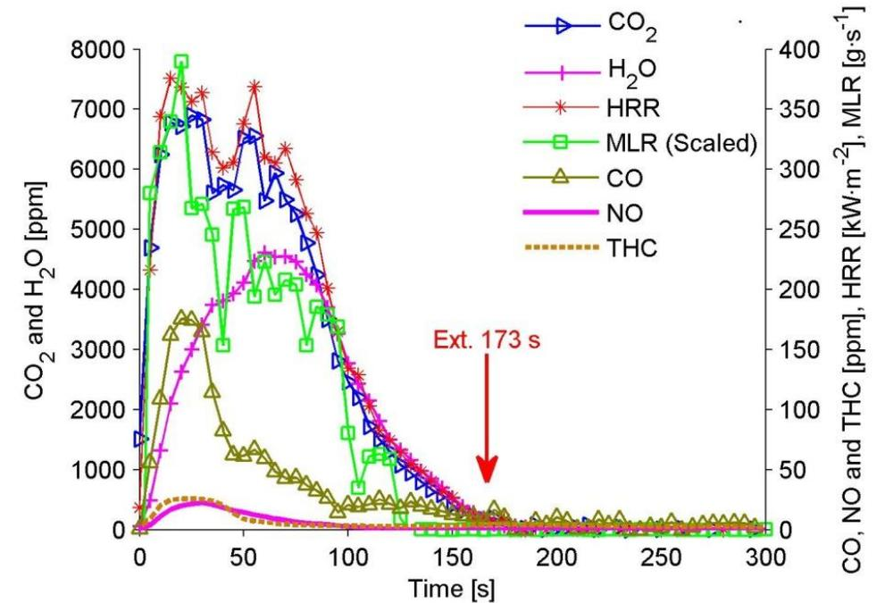
*Thermal decomposition of a PU Foam*
