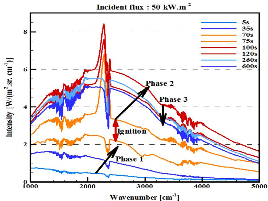
Radiative intensity emitted and reflected by a composite surface at  $50\text{ kW/m}^2$
