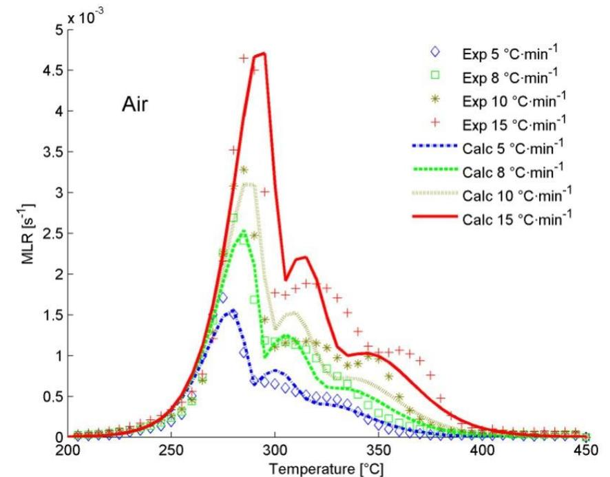
Comparison of numerical and experimental MLR curves in TGA
