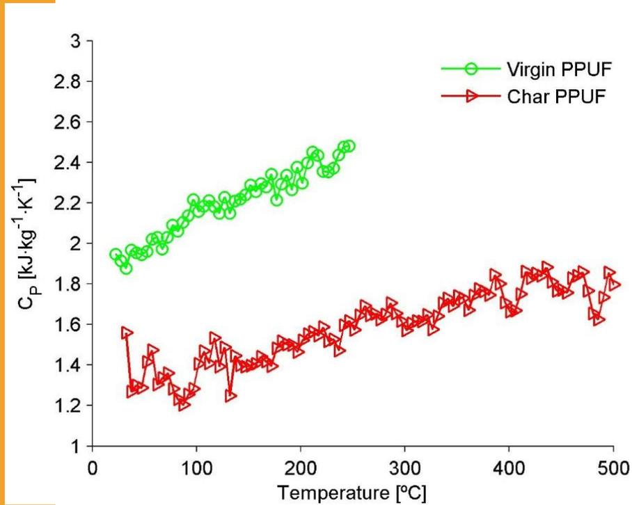
Example of  $C_p$  measurement of a PU Foam in DSC
