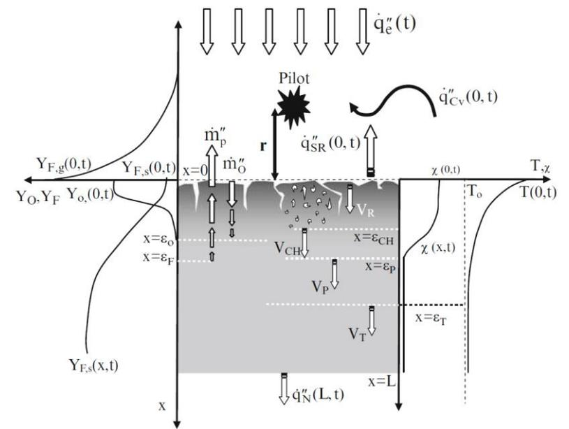
Simplified processus (1D) of thermal degradation of a solid – Torero, SFPE Handbook.
