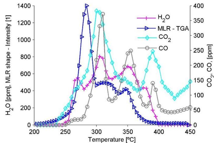
*Thermal degradation of a PU foam in TGA*
