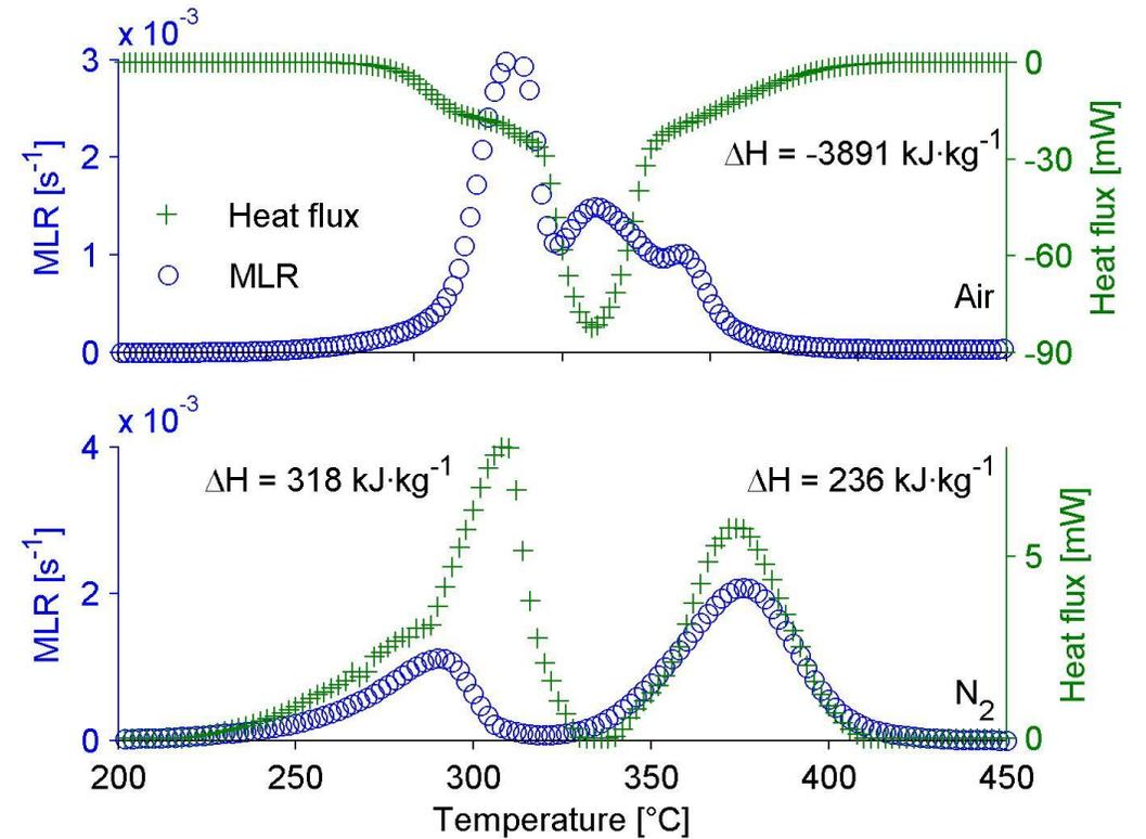
Example of  $\Delta H$  measurement of a PU Foam in DSC
