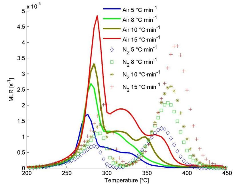
Thermal degradation of a PU foam in TGA
