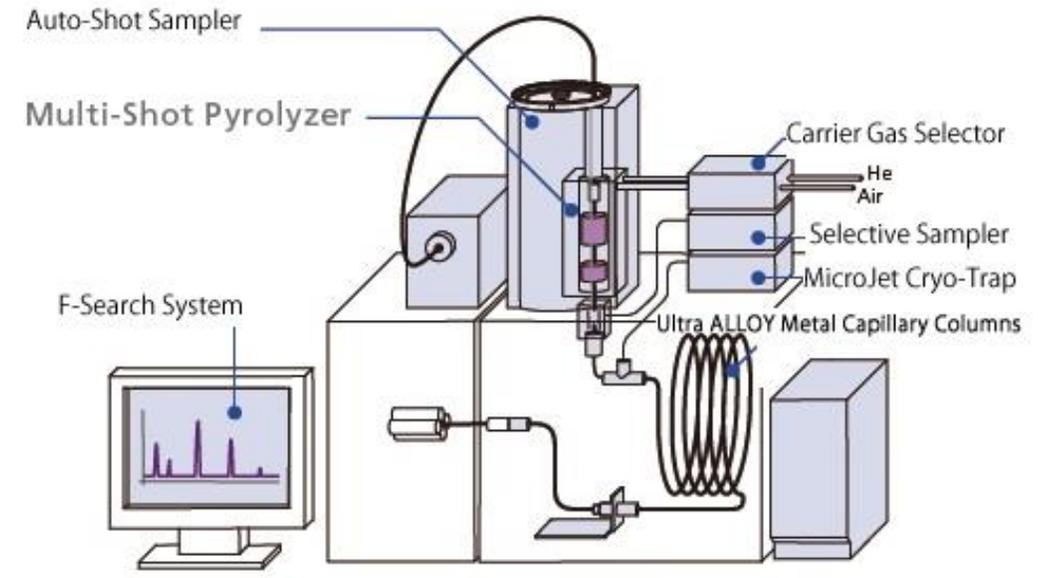
Py-GC/MS System (Multi-Shot Pyrolyzer and peripherals)
