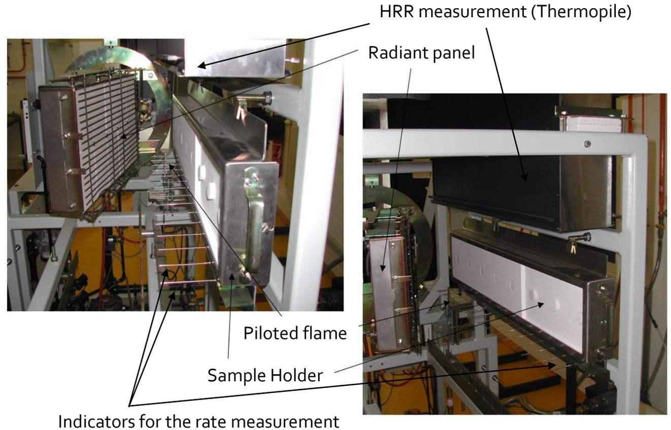
*IMO/LIFT Spread Of Flame Apparatus (ISO 5658)*
