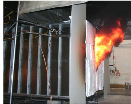
Experimental Study of the Effects of Fuel Type, Fuel ddistribution, and Vent Size on Full-Scale Underventilated Compartment Fires in an ISO 9705 Room
