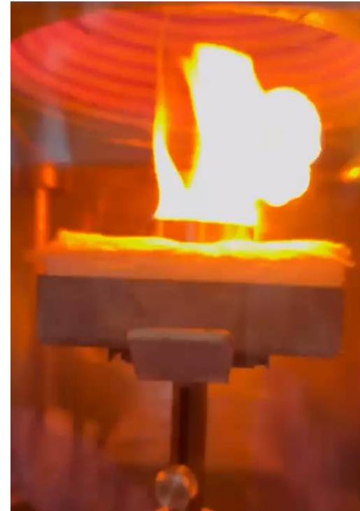
Low-intensity flame with intermittent flame flashes
