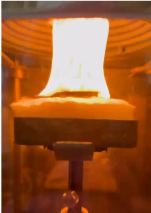
High-intensity flame Over flow and flame spread
