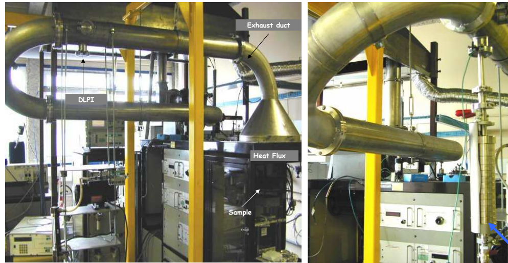
Low Pressure Impactor (DLPI) coupled with modified Cone Calorimeter
