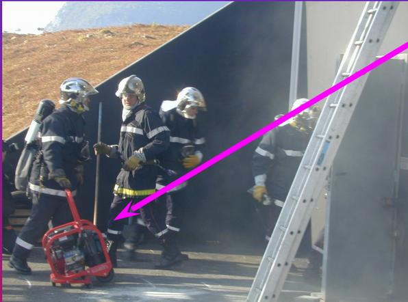
**E 1 - The fan is started in front of the door through which firemen will go in and out**
