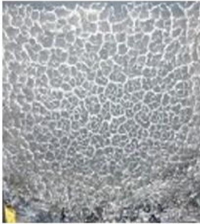
Plate 2. Photographs of the composite test samples after the 5 minutes fire resistance test (vertical configuration –face exposed to heat flux)
