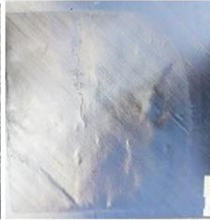
Plate 2. Photographs of the composite test samples after the 5 minutes fire resistance test (vertical configuration –face exposed to heat flux)
