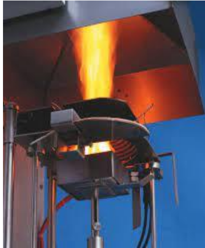
Horizontal cone calorimeter
