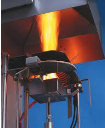
Horizontal cone calorimeter
